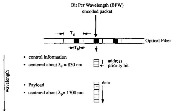
Fig. 3. Bit per wavelength encoding technique.
