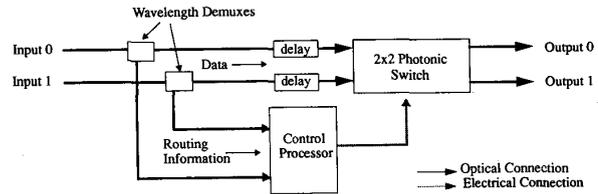
Fig. 4. 2 × 2 switch node architecture.
