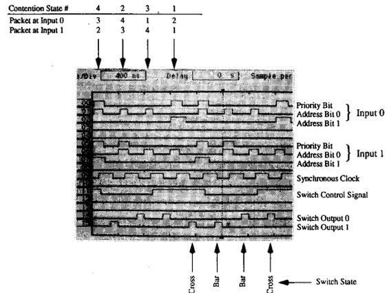
Fig. 6. Demonstration of self-routing with contention resolution.
