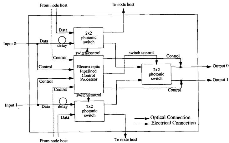
Fig. 2. A switching node for a photonic interconnect.
