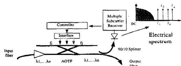
WJ6 Fig. 1. Schematic representation of the proposed configurations for channel equalization; the electrical spectrum after the photodiode is shown in the upper left corner.
