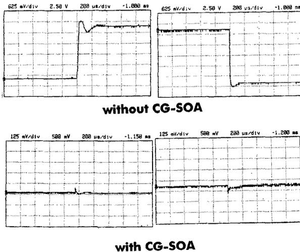
WJ4 Fig. 3. Surviving channel power when 3 channels out of 4 are dropped (left) or added (right). Time scale is 200  $\mu$ s/div. and the bottom line corresponds to zero optical power.
