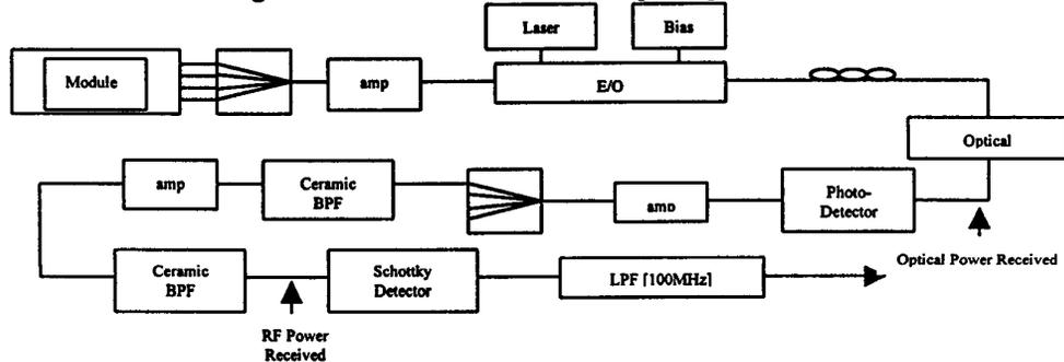
Figure 8. Complete OSCM Link Setup Diagram
