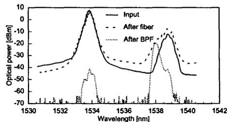
Figure 2. Optical spectrum at the input of the DSF, after the DSF and after the 0.2 nm BPF.
