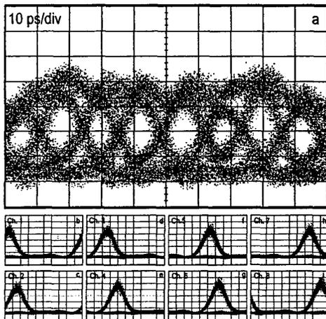
Figure 3. 80 Gbit/s eye diagram (a) and demultiplexed 10 Gbit/s channels (b-i).
