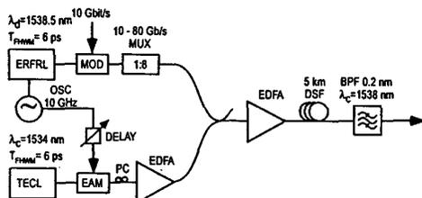
Figure 1. Experimental set-up. ERFL: erbium-doped fiber ring laser; MOD: LiNbO<sub>3</sub> modulator; MUX: passive 10 to 80 Gbit/s multiplexer; TECL: tunable external cavity laser; EAM: electroabsorption modulator; PC: polarization controller; EDFA: erbium-doped fiber amplifier; DSF: dispersion shifted fiber; BPF: optical band-pass filter.
