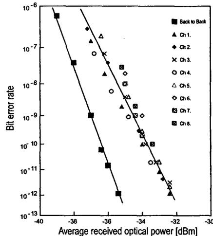
Figure 4. Bit-error rate measurements for 80 to 10 Gbit/s demultiplexing.
