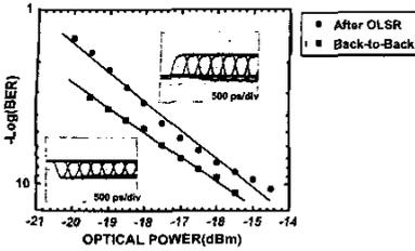
WO2 Fig. 3. Packet by packet bit-error-rates measured for back-to-back operation and for time domain contention resolution case.
