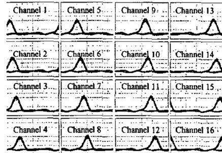
Fig. 4(b) Eye diagrams of 16 demultiplexed channels (Time 10ps/div)
