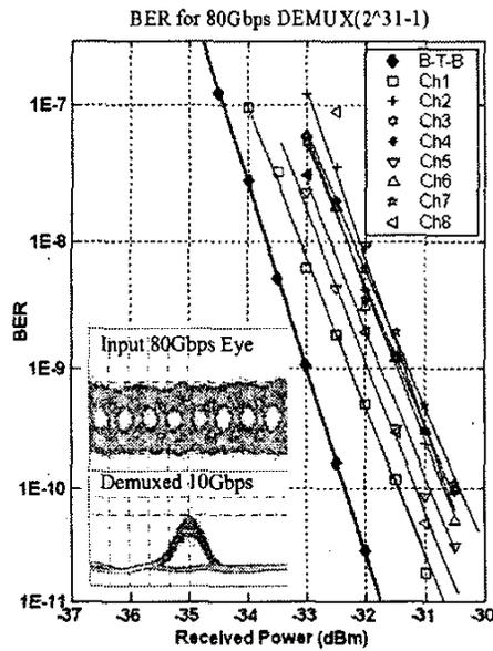
Fig. 3: Optical BER measurements for demultiplexing 80Gbps signal at 1546nm to 8 10Gbps channels
