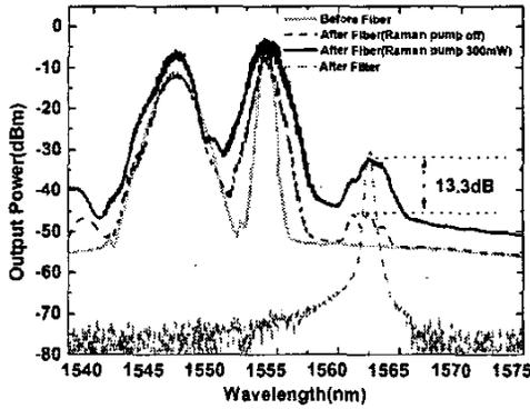
Fig. 2: Optical spectrum at various points of the DEMUX
