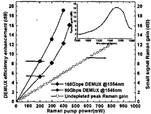
Fig. 5 FWM DEMUX efficiency enhancement measured at peak FWM component versus Raman pump power
