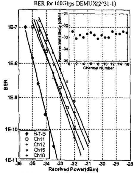
Fig. 4(a) Optical BER measurements for demultiplexing 160Gbps signal at 1554nm to 16 10Gbps channels
