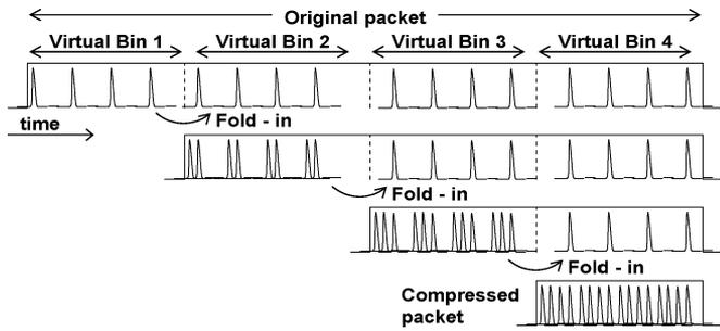
Fig. 2. Packet compression principle.
