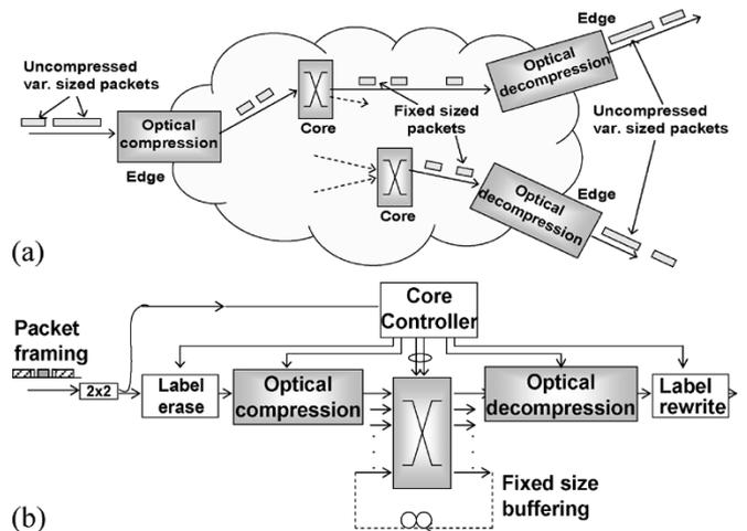
Fig. 1. (a) Compression and decompression placement at network edge and (b) at the core nodes.
