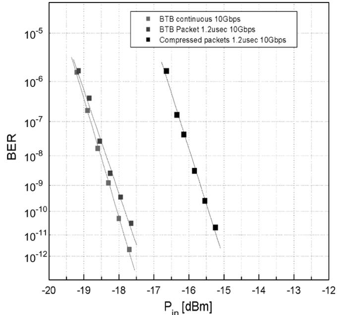
Fig. 5. BER measurement on compressed 1500-B packet at 10 Gb/s.
