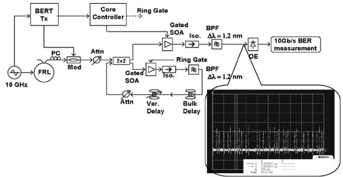
Fig. 3. Experimental setup for compression of variable sized packets from 2.5 to 10 Gb/s. (PC: Polarization controller. Attn: Attenuator. Iso: Isolator. BPF: Bandpass filter. FRL: Fiber ring laser.)
