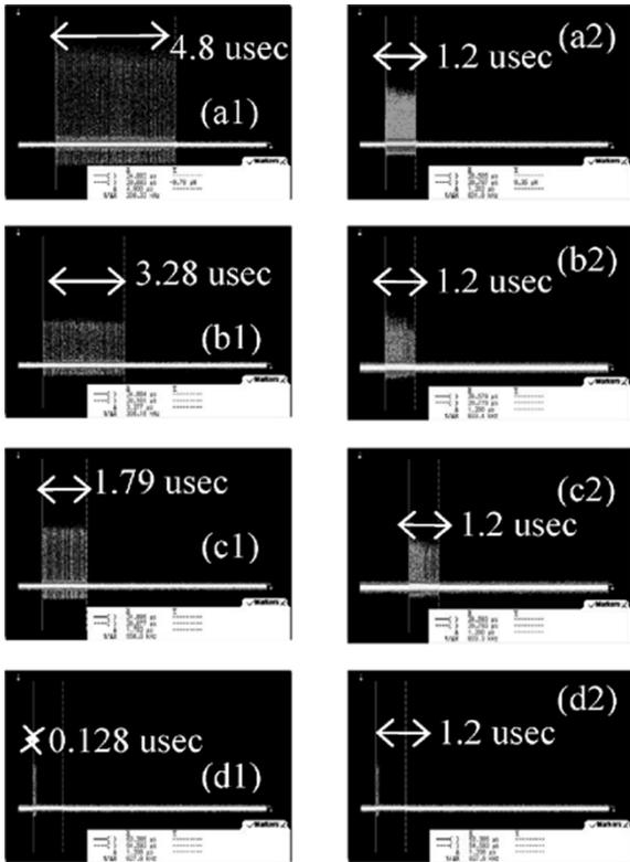
Fig. 4. (1) Uncompressed and (2) compressed packet traces taken at a  $1\text{-}\mu\text{s}/\text{div}$  scale for different input packet sizes. (a) 1500, (b) 1024, (c) 560, and (d) 40 B.
