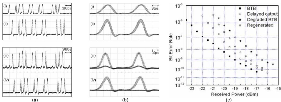
Fig. 4 (a) Waveforms and (b) eye diagrams of (i) input RZ packets and (ii) corresponding delayed RZ packets, (iii) degraded input RZ packets and (iv) corresponding regenerated delayed RZ packets; (c) BER results.
