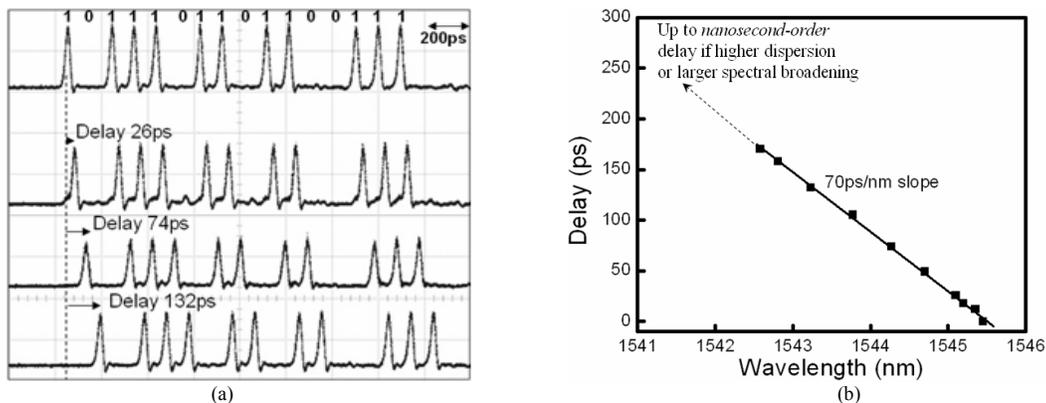
Fig. 3 (a) Oscilloscope traces showing time delay of the RZ packets varying with the center wavelength of the OBPF-2; (b) Linear function between time delay of the RZ packets and the center wavelength of the OBPF-2.
