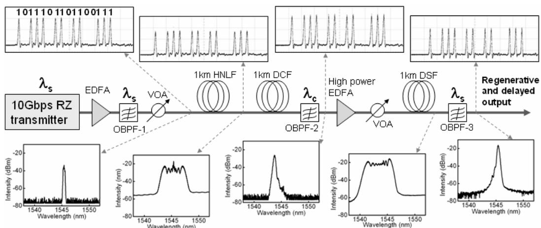
Fig. 1 Experimental setup (OBPF: optical bandpass filter; VOA: variable optical attenuator).
