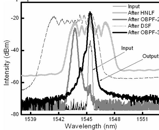
Fig. 2 Measured optical spectra of the 10Gbps RZ packets at different positions in the experimental setup.
