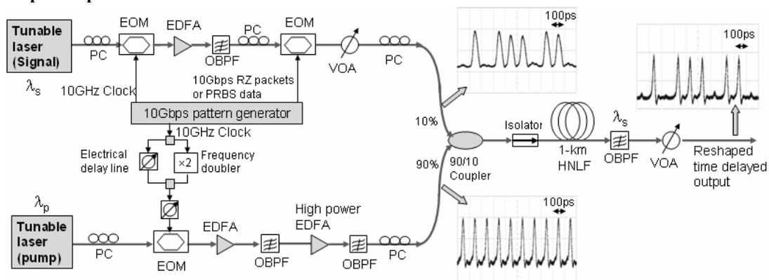
Fig. 1 Experimental setup (PC: polarization controller; EOM: E/O modulator; OBPF: optical bandpass filter; VOA: variable optical attenuator).
