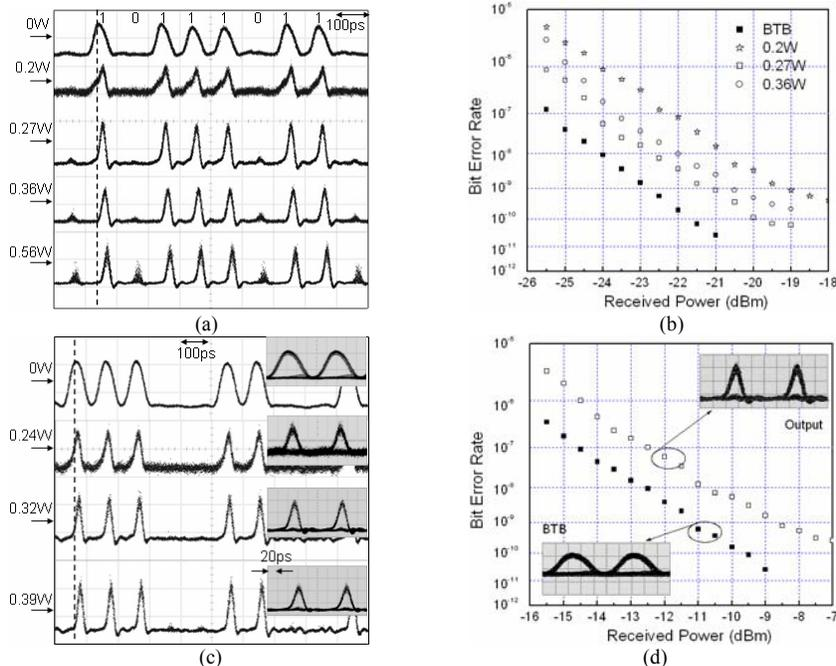
Fig. 3 Scope traces showing time delay of the signal varying with the pump powers when the signal is (a) RZ packet and (c) PRBS data; Corresponding BER results for (b) RZ packet and (d) PRBS data, respectively. Inset: corresponding eye diagrams.
