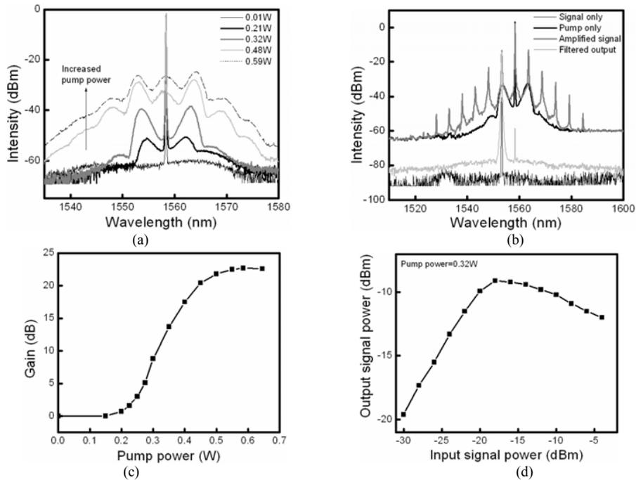
Fig. 2 (a) Measured OPA’s ASE spectra with variable pump powers; (b) Optical spectra measured at the OPA’s input/output before/after OBPF; (c) Measured gain versus variable pump powers; (d) Measured transfer function of the OPA.
