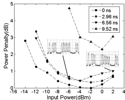
Figure 5: Input power dynamic range measurements.
