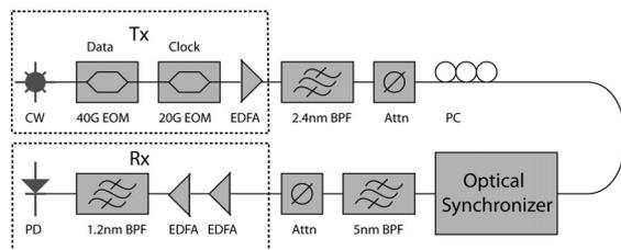
Figure 3: Experimental setup for BER measurements
