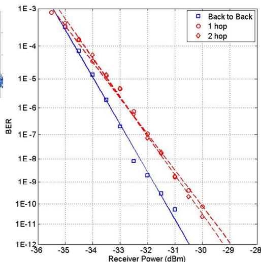
Fig.3(c) BER curves for input and converted signals
