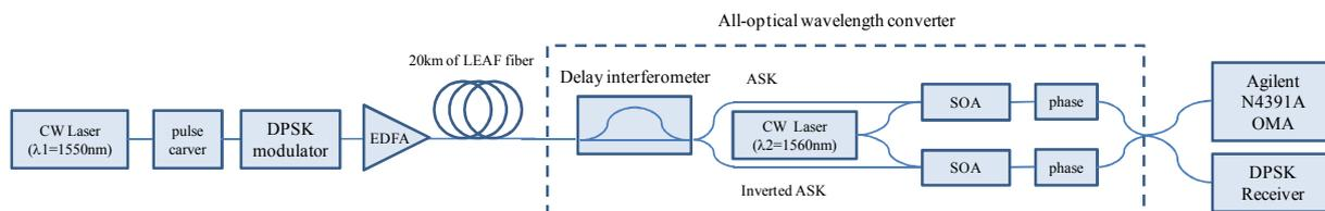
Fig.1(a) Experimental setup for investigating phase regeneration properties of all-optical DPSK wavelength converter
