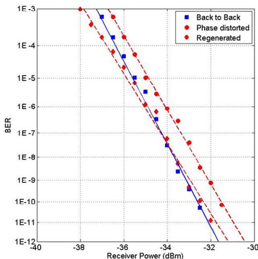
Fig.2(b) BER curves for input, phase distorted and regenerated signals.
