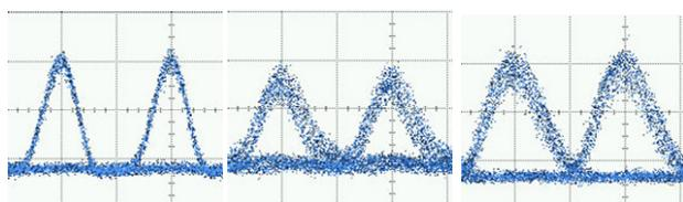
Fig.3(a) Eye diagrams at the output from single-ended DI in the receiver for input DPSK signals (left), first wavelength conversion (center) and second wavelength conversion (right).
