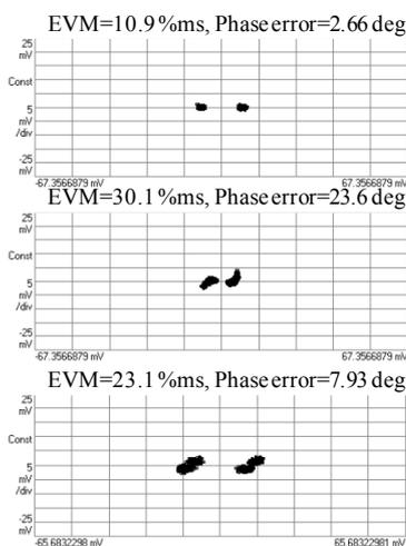
Fig.2(a) Constellation diagram for the input signal (top), phase distorted signal (middle), and regenerated signal (bottom).
