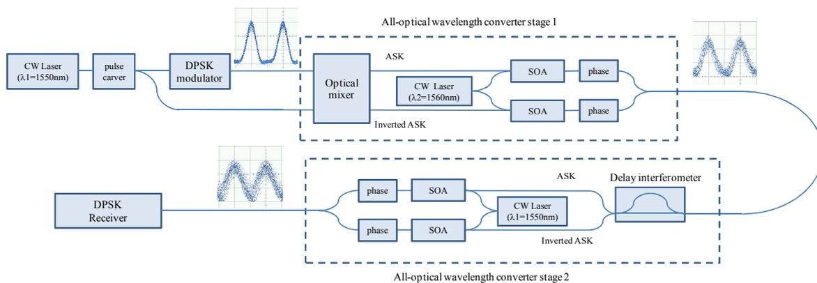
Fig.1(b) Experimental setup for cascading all-optical DPSK wavelength converters
