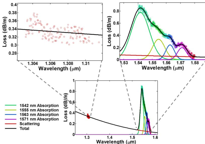
Fig. 4. Propagation loss (circles) vs. wavelength for a 40-nm-thick by 13- $\mu\text{m}$ -wide waveguide with bonded thermal oxide upper cladding. A 50 nm window function is applied in the spectral domain. The solid lines are fits of Gaussians (absorption loss) and a polynomial (scattering loss).
