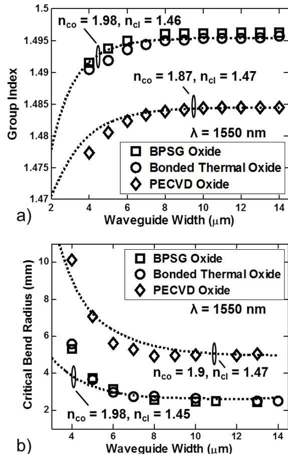
Fig. 2. a) Group index and b) critical bend radius data measured in 50 nm thick cores for the three approaches. Dashed lines are values simulated with the given refractive indices.
