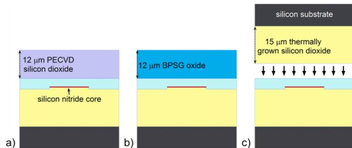
Fig. 1. Overview of the a) PECVD SiO<sub>2</sub>, b) reflowed BPSG, and c) bonded thermal oxide approaches compared in this work.
