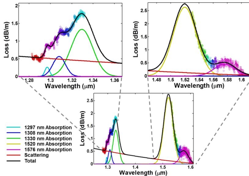
Fig. 3. Propagation loss (circles) vs. wavelength for a 50-nm-thick by 6.5- $\mu\text{m}$ -wide waveguide with PECVD oxide upper cladding. A 10 nm window function is applied in the spectral domain. The solid lines are fits of Gaussians (absorption loss) and a polynomial (scattering loss) to the data. The color key gives the loss type colors and the center wavelengths of the various Gaussian fits.
