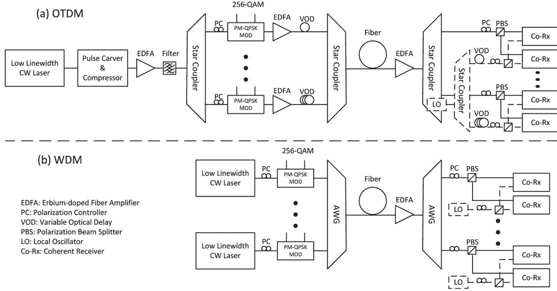
Fig. 1. Hypothetical 1 Tb/s links using Pol-MUX 256-QAM format, with (a)OTDM and (b)WDM.
