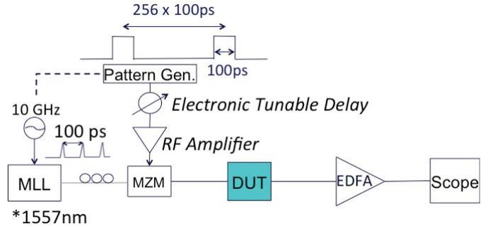
Fig. 6. Experimental set-up used to characterize delay configurations.
