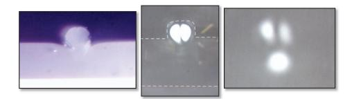
**Figure 4.2:** Microscope image of the facet and mode profiles as imaged with IR camera at the output of the "S" chip.
