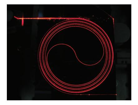
Figure 1.1: An example of a 1 meter-long waveguide fabricated out of the glasses  $Si_3N_4$  &  $SiO_2$ , illuminated with a red laser from an optical fiber (top-left). The time-delay corresponds to about 5 ns.[12]
