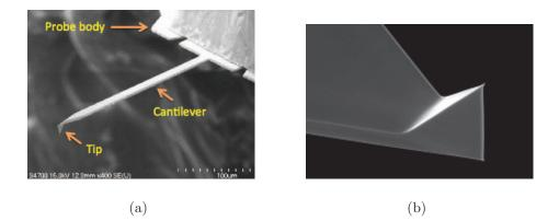
**Figure 3.3:** (a) SEM image of the AFM probe used for roughness measurements (Model: Olympus AC240TS) [29]. (b) Close-up of the tip (facing upwards) that makes contact with the sample surface. [30]
