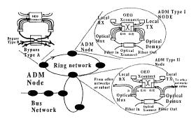
Fig. 4: The reconfigurable Add/Drop Multiplexer
