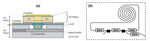
Fig. 1. (a) Schematic of the hybrid silicon amplifier cross-section [5]. (b) Schematic of the ULC-MLLD indicating the waveguides (black solid lines), couplers (black boxes) and chip boundary (dashed). The SOAs (grey) are realized as shown in (a).
