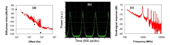
Fig. 3. (a) SSB phase noise plot of the first harmonic at 20 dBm RF power (red). The RF synthesizer phase noise (black diamonds) and analyzer noise floor (dashed line) are also indicated. (b) Time-domain trace obtained with a 53-GHz digital component analyzer. (c) Small-signal response of the free-running (continuous-wave) laser as measured by a 20-GHz Lightwave Component Analyzer. Signal is normalized to the lowest-frequency response.
