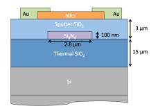
Fig. 2. Waveguide cross-section with the high aspect ratio core geometry of 2.8 um x 0.1 um.
