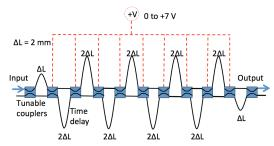
Fig. 1. Generalized lattice filter diagram with one-knob control for ease of bias. Colored boxes represent symmetric MZIs that serve the purpose of a tunable coupler.
