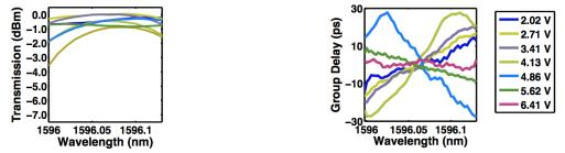
Fig. 3. Normalized filter transmission at different bias points
