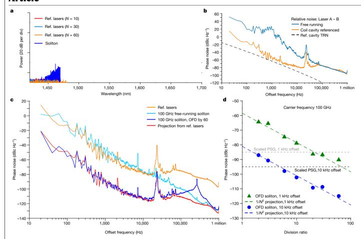
Fig. 3 | OFD characterization. a, Optical spectra of soliton microcombs (blue) and reference (Ref.) lasers corresponding to different division ratios. b, Phase noise of the frequency difference between the two reference lasers stabilized to coil cavity (orange) and the two lasers at free running (blue). The black dashed line shows the thermal refractive noise (TRN) limit of the reference cavity. c, Phase noise of reference lasers (orange), the repetition rate of
