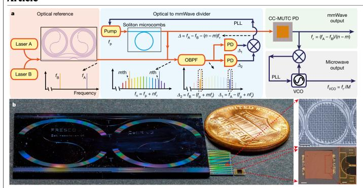
**Fig. 1** | **Conceptual illustration of integrated OFD. a**, Simplified schematic. A pair of lasers that are stabilized to an integrated coil reference cavity serve as the optical references and provide phase stability for the mmWave and microwave oscillator. The relative frequency difference of the two reference lasers is then divided down to the repetition rate of a soliton microcomb by feedback control of the frequency of the laser that pumps the soliton.
