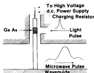
FIG. 1. Schematic of the microwave generator. A laser-triggered photoconductive switch is coupled to an X-band waveguide.
