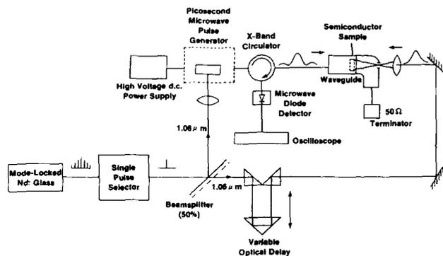
FIG. 3. Picosecond microwave pulse measurement. The microwave burst generated by a GaAs switch activated by a 30-ps,  $1.06\text{-}\mu\text{m}$  optical pulse coming from Nd:YAG mode-locked laser is gated by laser-induced reflectivity in a Ge wafer. The microwave reflectivity of the Ge is measured as a function of the time delay between the microwave and the optical bursts. The carrier recovery time in Ge is several microseconds so the time integral of the microwave burst can be generated.
