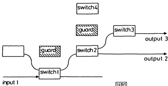
Fig. 1 Schematic layout: lower vertex of  $8 \times 8$   $\text{LiNbO}_3$  integrated-optic crossbar switch
