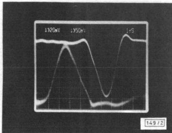
Fig. 2 Switching rise-time measurement: optical signal switched from output 2 (top trace) to output 3 (lower trace)
