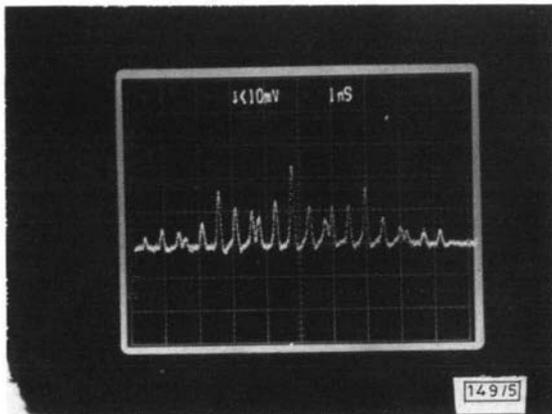
**Fig. 5** Autocorrelation function produced by shifting chip sequence (Fig. 4) through a matched fibre-optic tapped delay-line transversal filter
