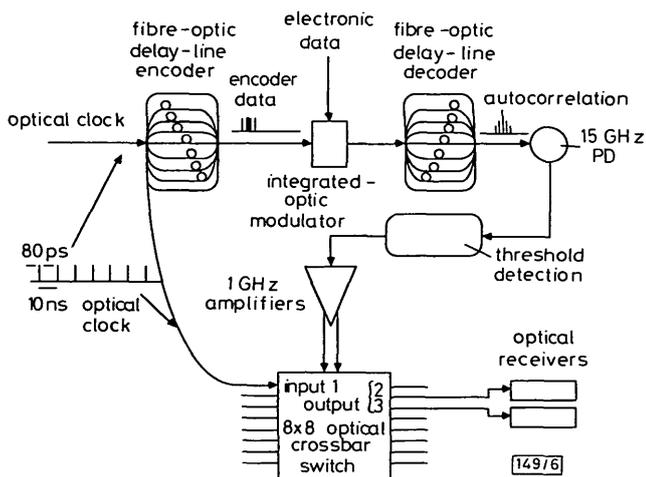
**Fig. 6** Schematic layout of optical self-routing experiment
