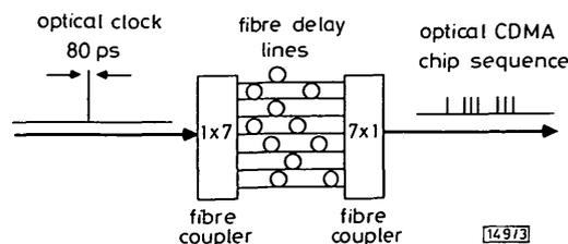
Fig. 3 Optical encoding of CDMA chip sequence using tapped fibre-optic delay-line processor
