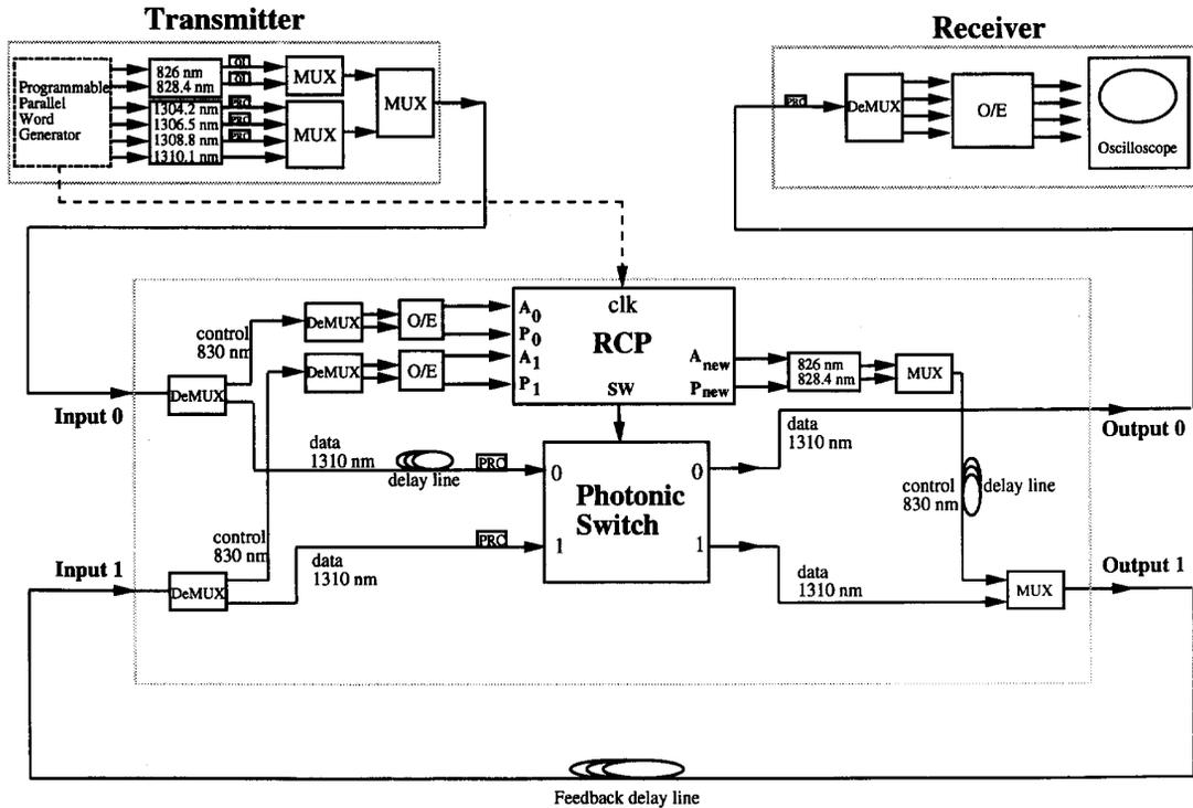
Fig. 3. Experimental setup used to demonstrate all-optical multihop photonic packet switching.
