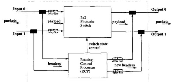
Fig. 1. A  $2 \times 2$  photonic switch building block.
