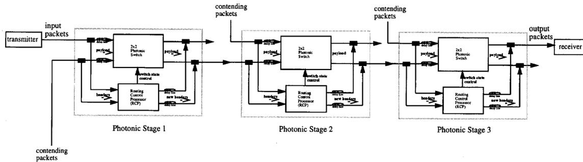
Fig. 2. Block diagram of multihop all-optical routing through three photonic packet switches.
