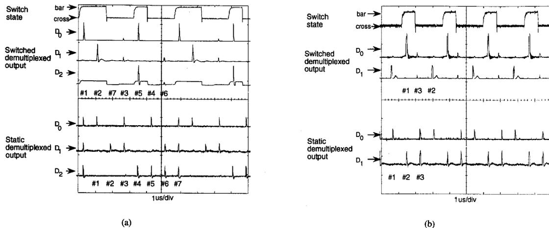
Fig. 4. Demultiplexed switch outputs.
