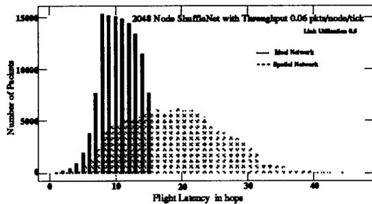
Figure 14: Flight Latency Histogram for a 2048-Node ShuffleNet with Spatial Nodes
