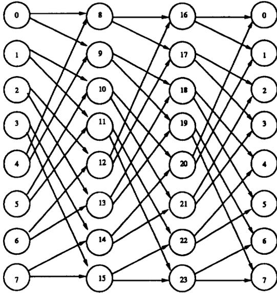
Figure 7: A 24 node ShuffleNet interconnect
