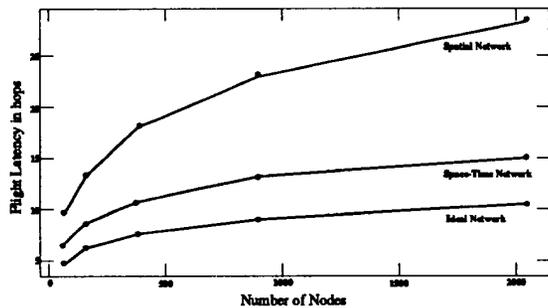
Figure 10: Variation of Maximum Flight Latency with Size
