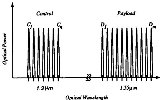
Figure 1: An example of Bit per Wavelength Encoding
