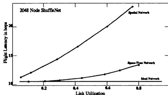
Figure 12: Flight Latency vs. Link Utilization for a 2048-Node ShuffleNet
