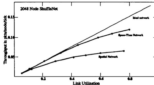
Figure 13: Throughput vs. Link Utilization for a 2048-Node ShuffleNet
