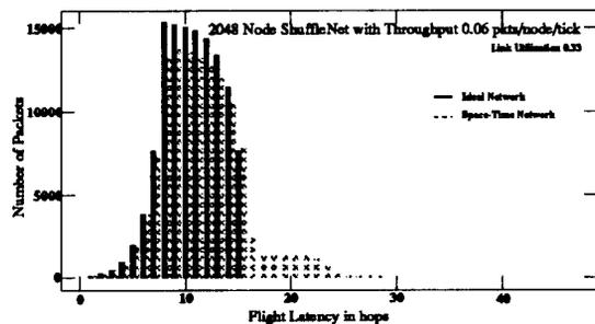
Figure 15: Flight Latency Histogram for a 2048-Node ShuffleNet with Space-Time Nodes
