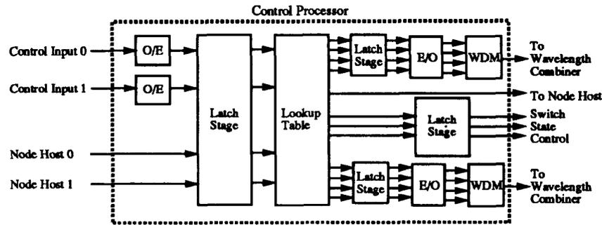
Figure 5: Block diagram of a parallel pipelined switch control processor
