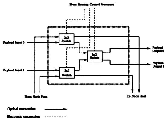
Figure 4: The Photonic Switch
