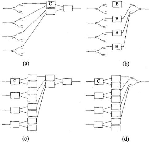
Fig. 1. Four switch architectures investigated are: (a) asac, (b) aspc, (c) psac, and (d) gaa. Power crosstalk for directional coupler switches are indicated by  $C$  and the gate array element extinction ratio is indicated by  $E$ . Passive splitters and combiners are shown as  $Y$  branched waveguides.
