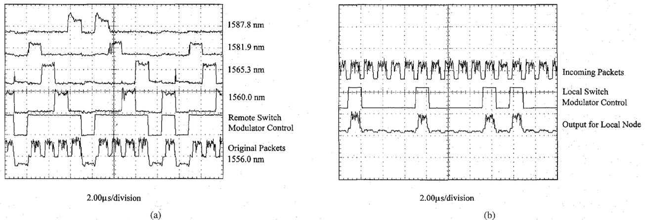
Fig. 2. (a) Remote port routing function: Traces 1-4 are wavelength converted and switched packets, Trace 5 is remote modulator control signal, Trace 6 is monitor of 512-b payloads at original wavelengths. (b) Local port routing function: upper trace is input packets, middle trace is modulator control, lower trace is local port packets.
