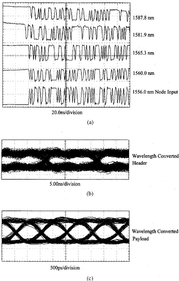
Fig. 3. (a) Wavelength conversion of original payload (lower trace) to four different wavelengths (1587.8 nm, 1581.9 nm, 1565.3 nm, and 1560 nm from top down). (b) Eye diagram of wavelength converted demodulated header. (c) Eye diagram of wavelength converted baseband.
