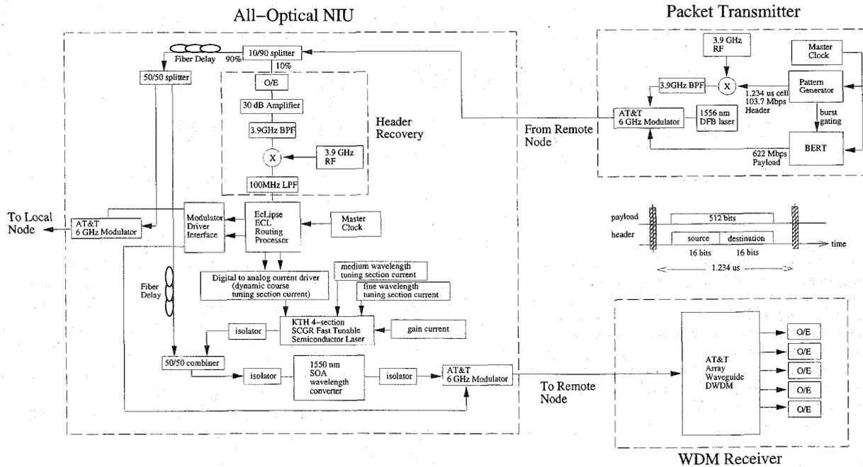
Fig. 1. Network node architecture includes network interface unit (NIU), local host, and baseband/optical-subcarrier-multiplexed transmitter/receiver.
