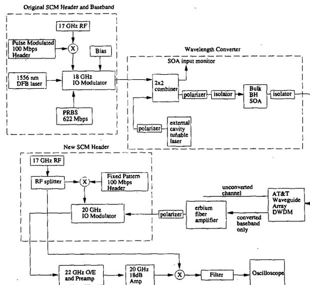
**WG6** Fig. 1. Experimental setup of all-optical simultaneous wavelength conversion and SCM header removal and generation.
