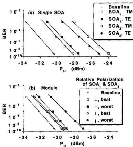
**WG5** Fig. 3. (a), (b) The BER measurement of the wavelength shifted signal for single-SOA and two-SOA wavelength shifter. The power parameters are the same as Fig. 2.
