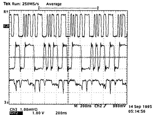
**WG6 Fig. 3.** Measurement of cross talk between demodulated original header and demodulated new header. Top trace is header data, middle trace is demodulated new header, lower trace is demodulated original header.
