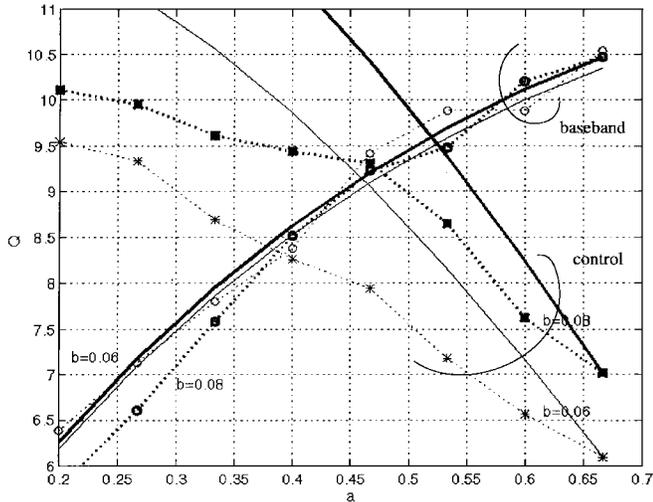
Fig. 3. Experimental (point and dashed lines) and analytical (solid lines) measurement of  $Q_p$  and  $Q_h$  as a function of the normalized baseband signal amplitude  $a$  for two different values of the normalized control signal amplitude  $b$ .
