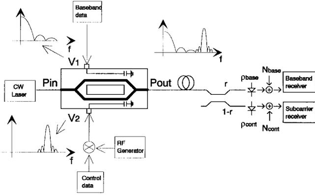
Fig. 1. Schematic of our OSCM architecture based on differential external modulator, together with a schematic of a generic baseband and subcarrier receiver.
