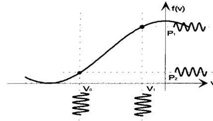
Fig. 2. Nonlinear mapping of payload and header modulation by Mach-Zehnder interferometric modulator illustrating operating end points for baseband data and binary quiescent operating points for subcarrier multiplexed control channel.
