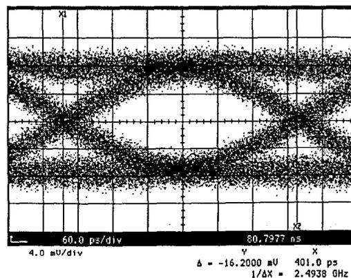
Fig 3 (a) Experimental Results: Payload eye diagram
