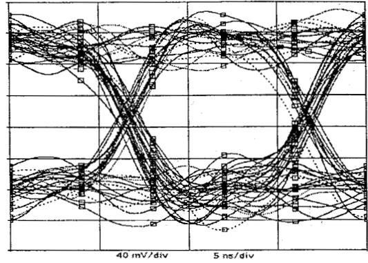
Figure 6. Header eye diagram with coherent detection scheme
