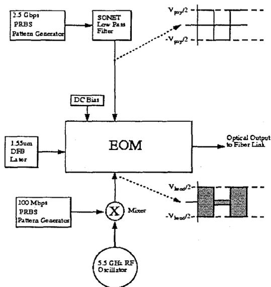
Fig. 1 (a) Experimental Link: Transmitter and EOM
