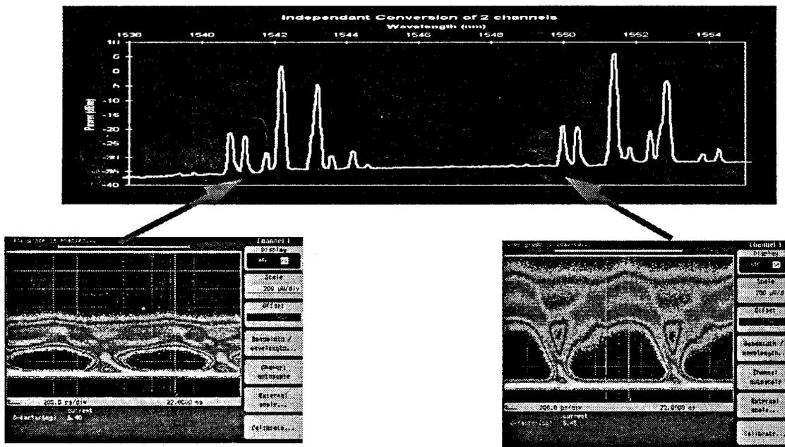
Figure 2: Optical spectrum at the SOA output and eye diagrams of converted signals at 1GBps.
