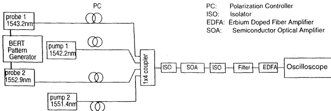
Figure 1: Setup of the two independent pump/two probe four wave mixing experiment
