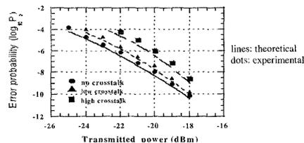
A 0.8 nm-misalignment of one of the transmission channels during the demonstration did not introduce any power penalty, showing the detuning tolerances of the AOTS.
