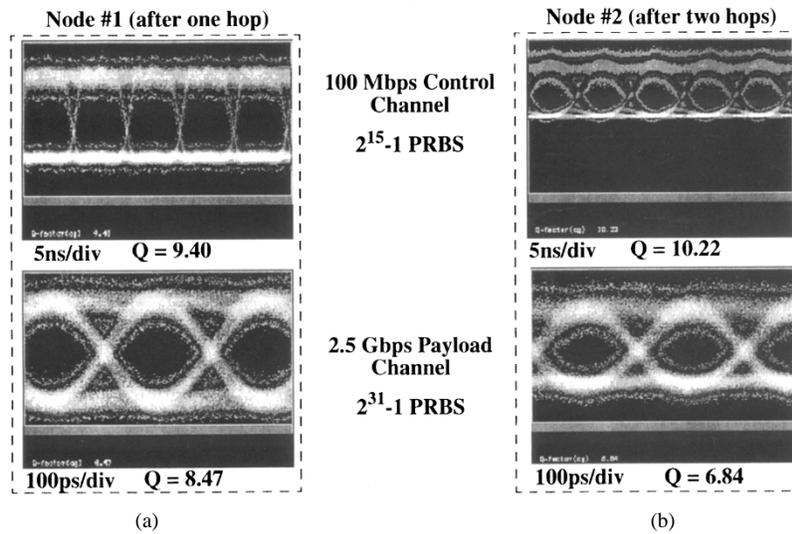
Fig. 11. Eye diagrams of the recovered payload and header channels for packets dropped at (a) node #1 and (b) node #2. The payload channel consists of a  $2^{31} - 1$  PRBS pattern. The header channel consists of a  $2^{15} - 1$  PRBS pattern.
