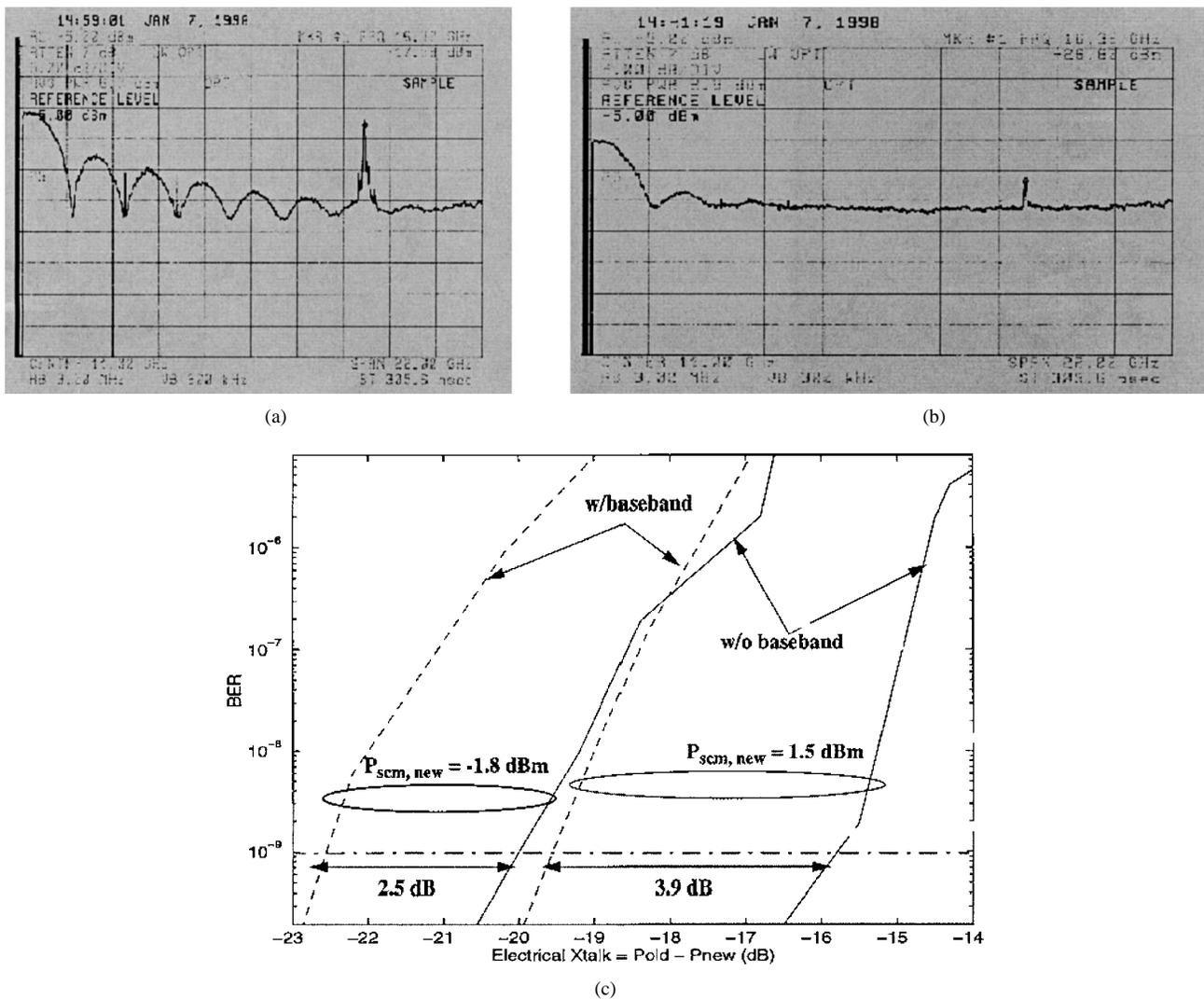
Fig. 12. Demonstration of header replacement using a XGM SOA-WC. (a) Input RF power spectrum, (b) wavelength converted power spectrum with suppressed subcarrier header, and (c) BER measurements of recovered baseband and new header in the presence of interfering unsuppressed old header.
