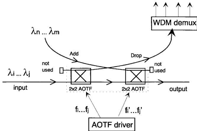
Fig. 6. Schematic of the dilated  $2 \times 2$  AOTF switch and the optical demux.
