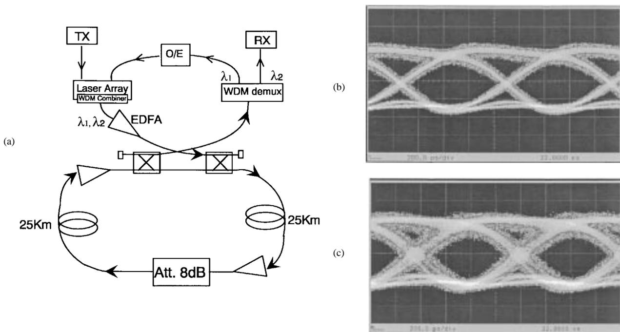
Fig. 14. (a) Experimental setup of two hop bypass with 2R OEO regeneration and wavelength translation, (b) eye diagram after first hop, and (c) eye diagram after second hop.
