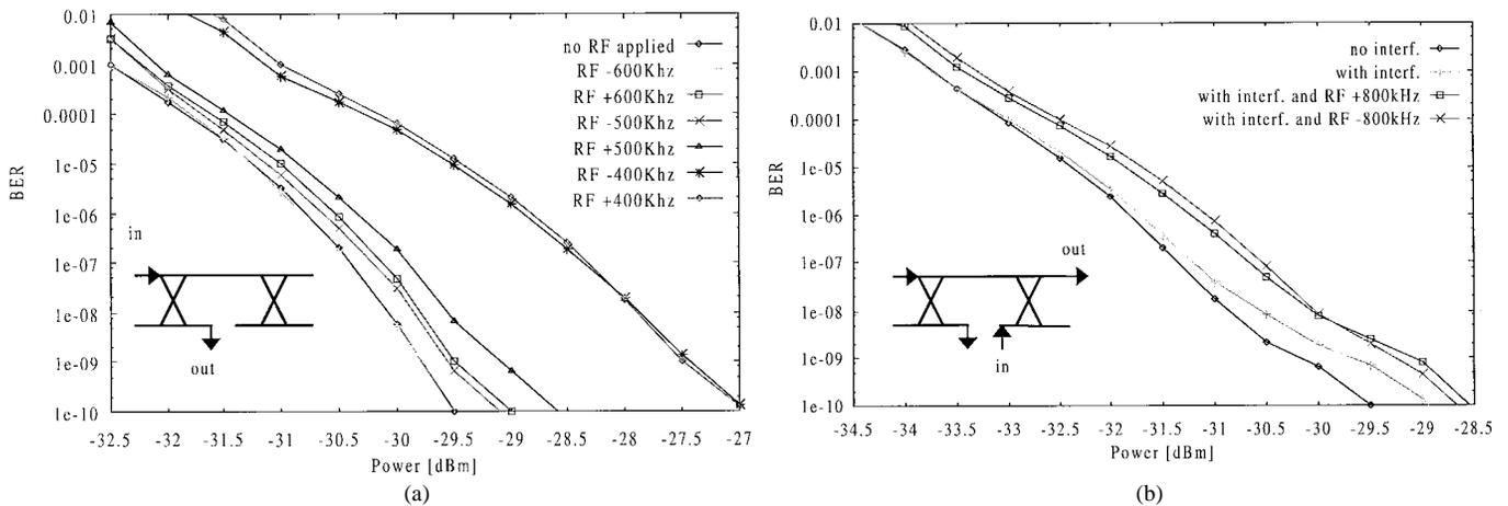
Fig. 8. BER measurement on the dilated AOTF in the presence of multiple RF frequencies: (a) drop port and (b) add port.
