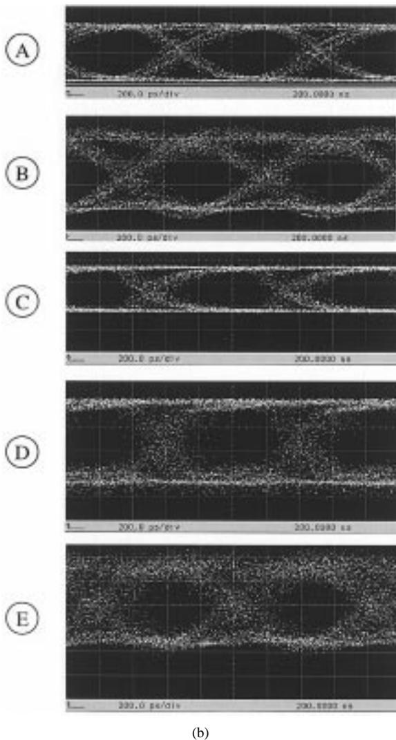
Fig. 16. (*Continued.*) Schematic of three-node multihop WDM add/drop lightpath experimental demonstration. Dark lines indicate physical connections and light grey lines indicate lightpath. Eye diagrams at various points in network are indicated by A, B, C, D, and E. The optical power spectrum is shown in the center insert F.
