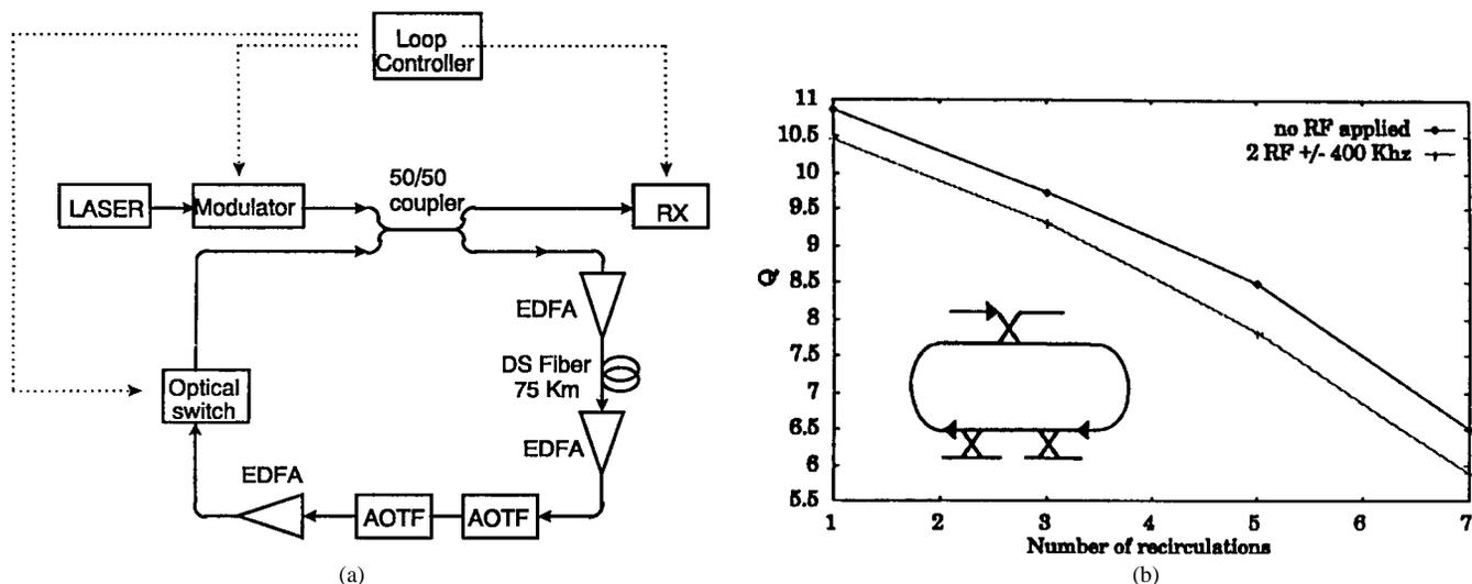
Fig. 15. (a) Experimental setup of seven-hop multichannel optical bypass demonstration and (b)  $Q$  as a function of the number of recirculations.
