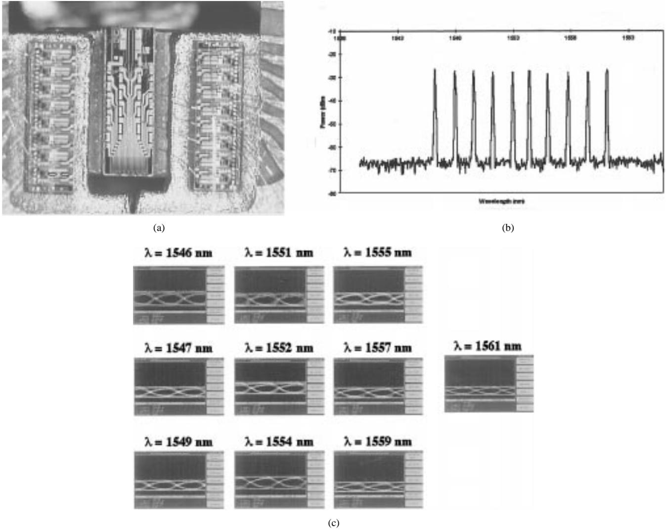
Fig. 10. (a) Packaged multiwavelength laser array transmitter, (b) optical output spectrum of ten wavelengths, and (c) 2.5 Gbps eye diagrams for all ten channels.
