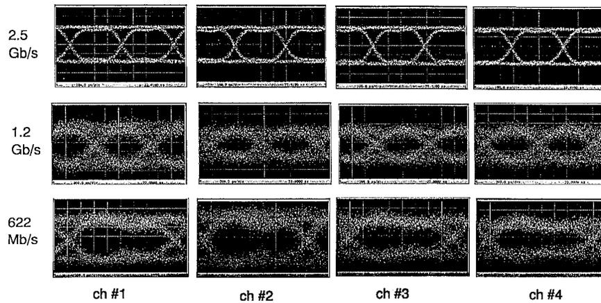
Fig. 13. Eye diagrams illustrating bit rate transparency for 622 Mbps, 1.2 Gbps, and 2.5 Gbps.
