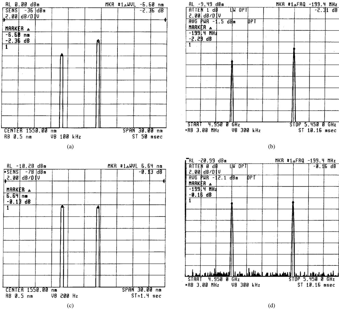
Fig. 9. Two channel equalization using measured subcarrier signal levels: (a) optical input spectrum, (b) electrical input spectrum, (c) optical spectrum after equalization, and (d) electrical spectrum after equalization.
