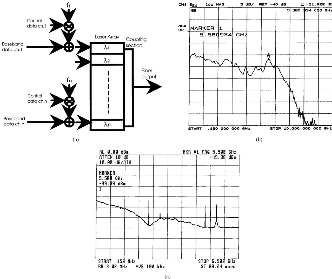
Fig. 11. (a) Schematic for SCM multiwavelength laser array transmitter; (b) frequency response of the laser array on the subcarrier port; and (c) output spectrum on one channel of the laser array when a 2.5 Gbps baseband signal and a 5.5 GHz 100 Mb/s subcarrier signal are applied.
