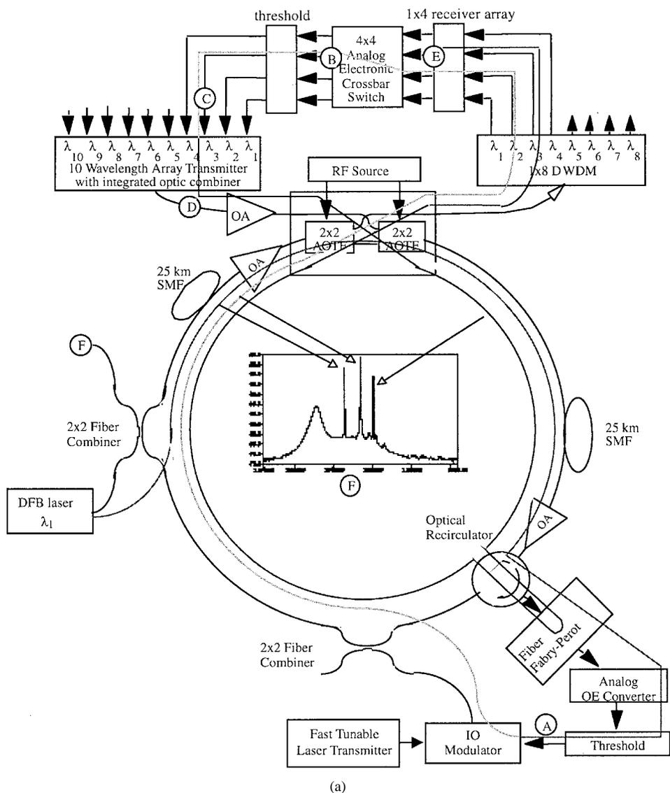
Fig. 16. Schematic of three-node multihop WDM add/drop lightpath experimental demonstration. Dark lines indicate physical connections and light grey lines indicate lightpath. Eye diagrams at various points in network are indicated by A, B, C, D, and E. The optical power spectrum is shown in the center insert F.
