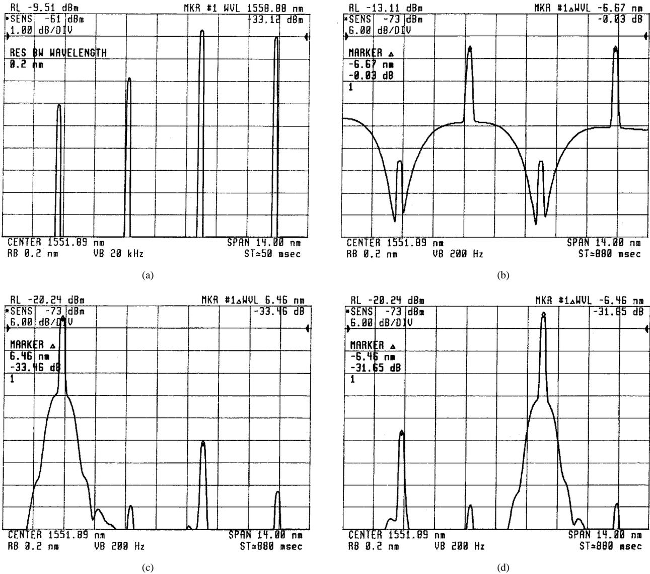
Fig. 7. Demonstration of WDM multichannel add/drop using dilated AOTF 2 × 2 switch: (a) dilated AOTF input, (b) dilated AOTF output, (c) dropped wavelength 1, and (d) dropped wavelength 3.
