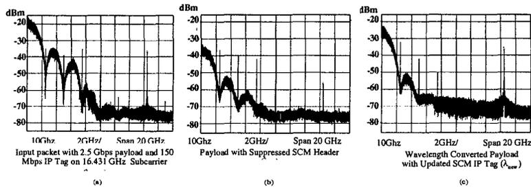
Figure 3. RF power spectrum for (a) packet input to tag switching setup, (b) output of XGM-WC showing SCM header suppression and (c) remodulated output of tag switching with wavelength conversion.
