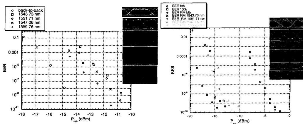
Figure 4. On Left: Measured transmission BER for output baseband payload for four different wavelengths and back-to-back. On right: Measured BER for recovered SCM Tag at transmitter and after Tag switching for four different wavelengths.
