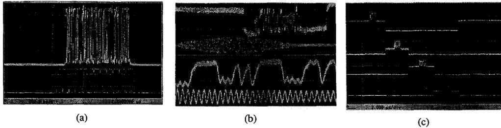
Figure 2. (a) Parallel received 2.5 Gbps payload (upper trace) and 150 Mbps Tag/Header (lower trace). (b) Recovered Tag/Header clock and data. (c) Output of Tag Switching experiment illustrating noninverting wavelength conversion at the packet rate between four output wavelengths.
