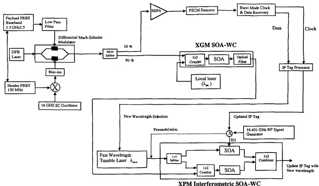
Figure 1. Architecture of WDM Optical IP Tag Switching Experiment using cascaded wavelength converters and optical subcarrier multiplexed tags.
