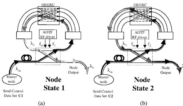
Fig. 2. Graphical representation of (a) Node State 1 and (b) Node State 2. Thin lines show physical connections while thick lines show signal path on different wavelengths.
