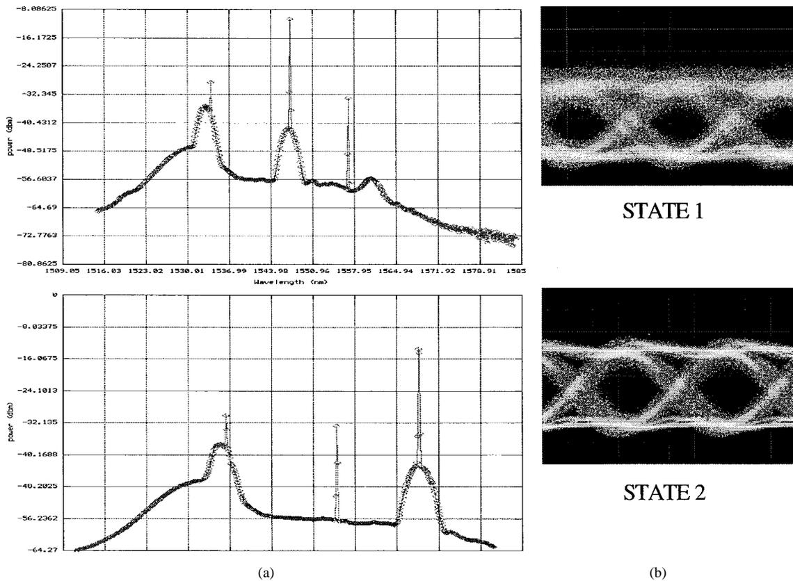
Fig. 3. Remote reconfiguration of multichannel ADM node. Upper traces are for State 1 and lower traces for State 2. (a) Optical spectrum at the ADM output port and (b) measured eye diagram at optical output port.
