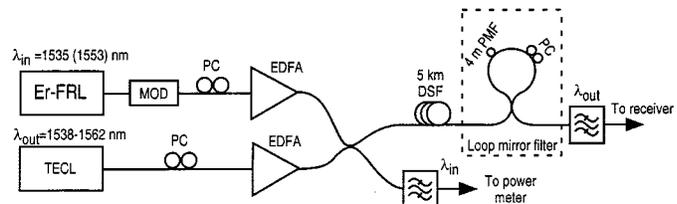
Fig. 1. Experimental setup of the XPM wavelength converter. Er-FRL: fiber ring laser; TECL: tunable external cavity laser; MOD: Mach-Zehnder modulator; EDFA: erbium-doped fiber amplifier; PC: polarization controller; PMF: polarization maintaining fiber; DSF: dispersion shifted fiber.
