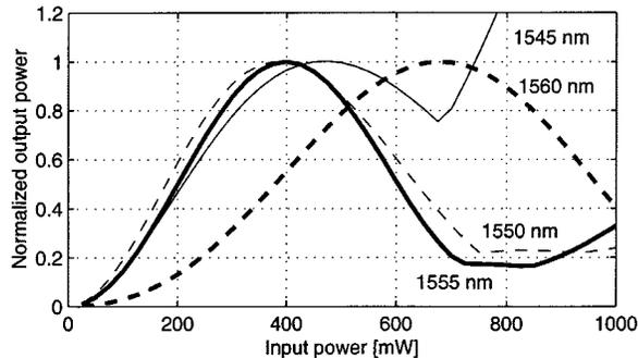
Fig. 5. Simulation of the transfer function for 2-ps input pulses at 1535 nm using a highly nonlinear DSF, aiming at 160 Gb/s.
