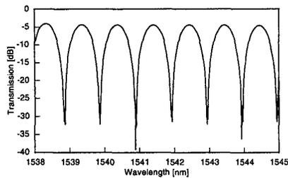
**Figure 2.** Transmission through the loop mirror filter.
