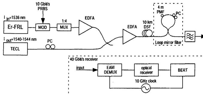
**Figure 1.** Experimental set-up of the XPM wavelength converter. Er-FRL: Fiber ring laser; MOD: LiNbO<sub>3</sub> modulator; EDFA: Erbium-doped fiber amplifier; PC: polarization controller; PMF polarization maintaining fiber; EAM: electro-absorption modulator; BERT: bit-error rate test set.
