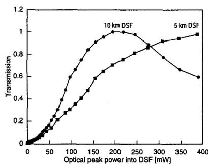
**Figure 4.** Transmission versus input peak power for the wavelength converter using a 10 km and 5 km DSF.
