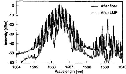
**Figure 3.** Output optical spectrum of original data and wavelength converted signal before and after the filter.
