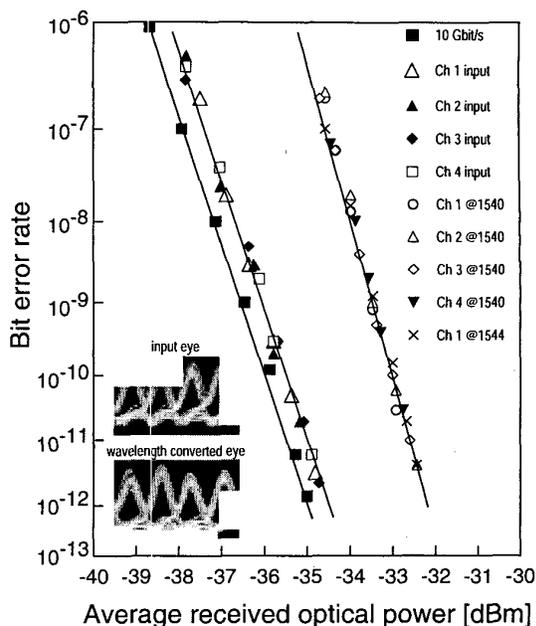
Figure 5. Bit-error rate measurements for wavelength conversion of 40 Gbit/s data from 1536 nm to 1540 nm and 1544 nm.
