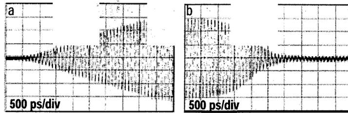
Figure 2. Beginning (a) and end (b) of the electrical drive signal to the ring laser.
