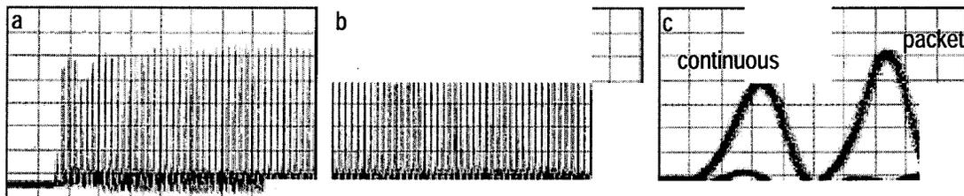
Figure 3. Optical output from the laser. a and b shows the beginning and the end of the packet, and c shows the 10 ps pulse from the laser in continuous mode and in packet mode.
