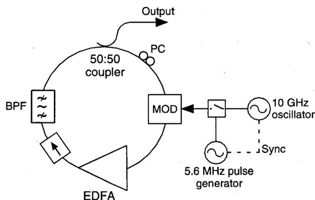
Figure 1. Experimental set-up. MOD:  $\text{LiNbO}_3$  modulator; EDFA: erbium-doped fiber amplifier; BPF: 0.6 nm optical band-pass filter; PC: polarization controller.
