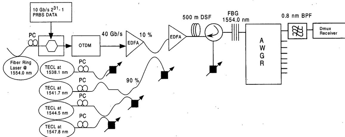
Fig. 1. Experimental setup to simulate a node in the proposed broadband architecture
