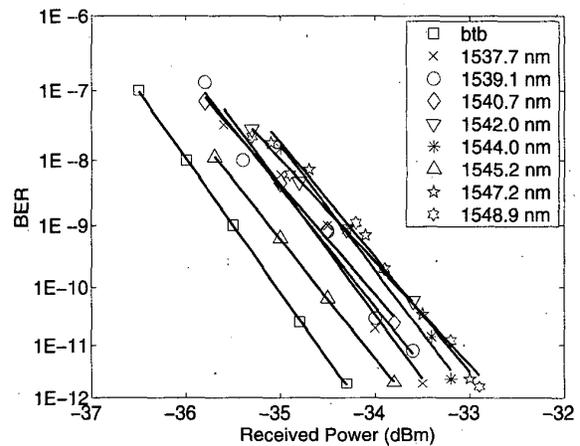
Fig. 5(b). BER curves for 1 input channel (back-to-back) and 1 channel for each of the 8 broadcast wavelengths
