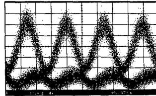
Fig. 4(b). Output 40 Gbit/s eye at 1545.2 nm
