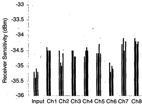
Fig. 5(a). Receiver sensitivities for the 32 - 10 Gbit/s output OTDM channels and the 4 10 Gbit/s input OTDM channels
