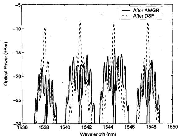
Fig. 3. Optical Spectrum before and after the AWGR
