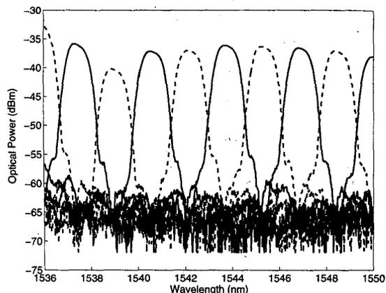
Fig. 2. Pass band of all the ports of the AWGR in the region of interest
