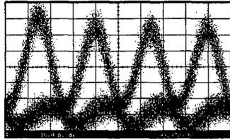
Fig. 4(a). Input 40 Gbit/s eye at 1554.0 nm
