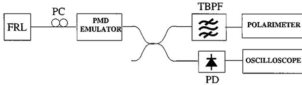
Fig. 4. Experimental setup. FRL: Fiber ring-laser. TBPF: Tunable bandpass filter. PC: Polarization controller. PD: Photodetector.
