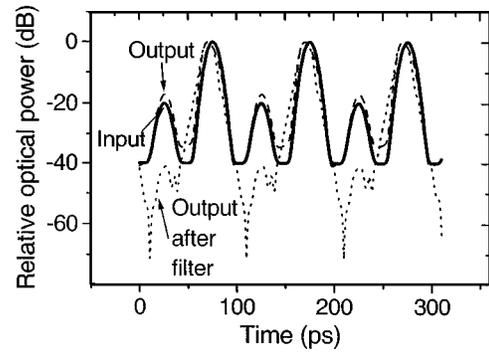
Fig. 3. Simulated pulse train at input (solid) of SOA, after SOA (dashed), and after SOA + BPF (dotted).
