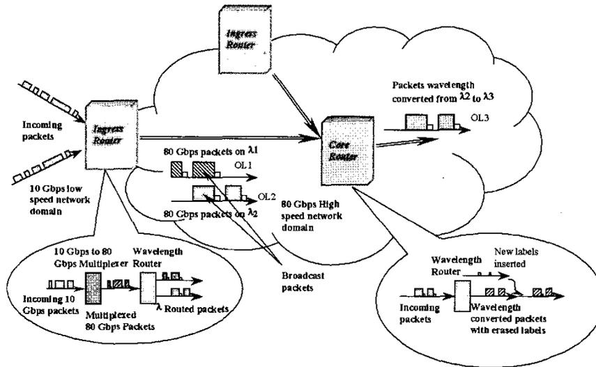
Figure 1. AOLS system architecture example with ingress, core and egress routers.
