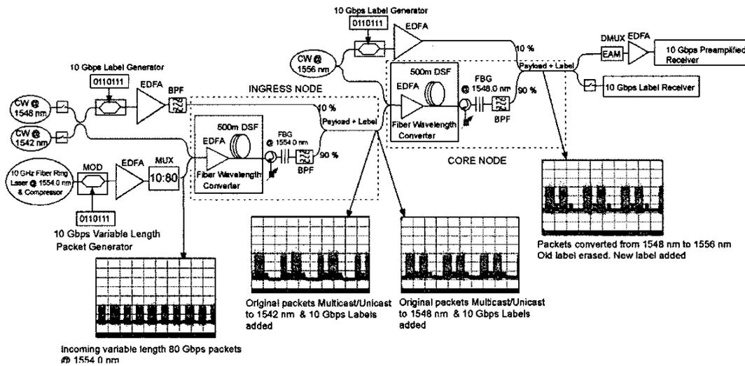
Figure 2. Experimental setup for demonstration of 80Gb/s packet/10Gb/s optical label multihop AOLS
