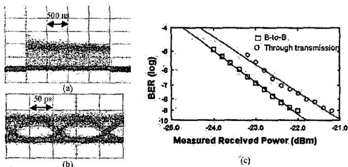
Fig. 4: a) Waveform of the 2-us data burst sent from the slave node and received at the master node, b) A zoom-in eye diagram of the 10-Gb/s signal, c) BER measurements.
