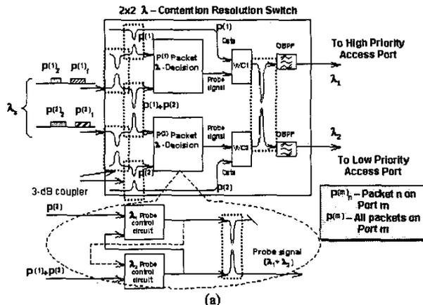
Fig. 2 (a) Structure and operation principle of  $2 \times 2$   $\lambda$ -contention resolution switch (b) Timing diagram for probe signals generated
