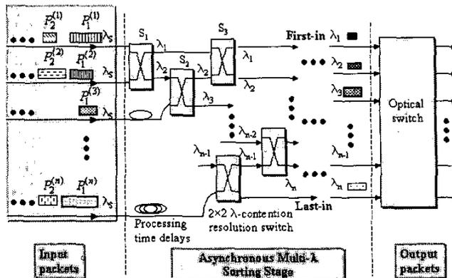
Fig. 1 Proposed all-optical sorting scheme for multiple packets
