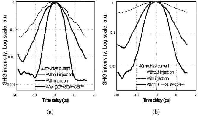
Fig. 4. Autocorrelation traces for output pulses without injection, with injection and after SOA+OBPF at different bias current. (a) 60 mA. (b) 40 mA.
