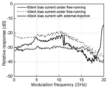
Fig. 2. DBR-LD frequency response under free-running and external injection.
