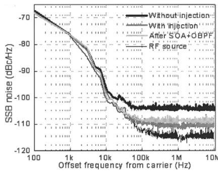
Fig. 5. SSB noise spectra measured for the RF source, 20-GHz pulses without injection, with injection, and after SOA+OBPF at 60-mA bias current of DBR-LD.
