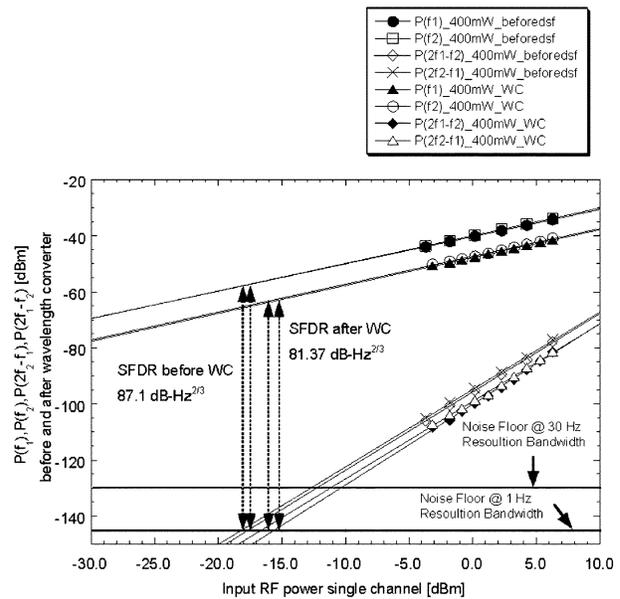
Fig. 3. SFDR measurement before and after DSF for average optical power of 400 mW.
