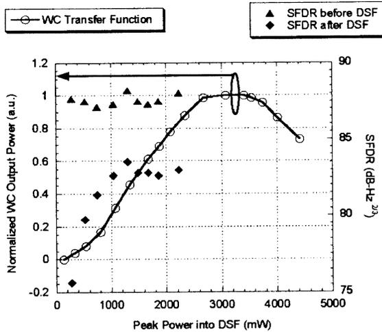
Fig. 4. Measurement of the link SFDR with and without the wavelength converter.
