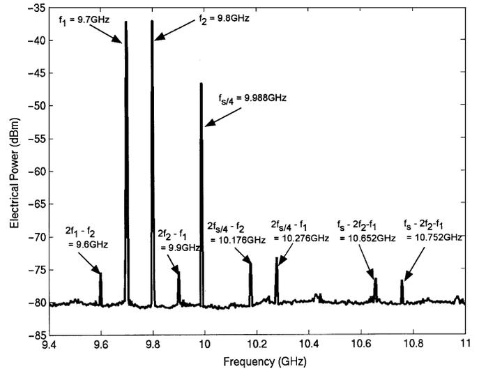
Fig. 2. Example measured RF power spectra for time sampled two-tone signal.
