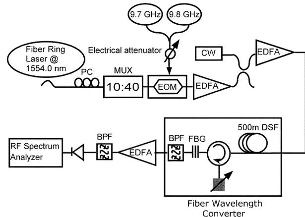
Fig. 1. SFDR measurement setup.
