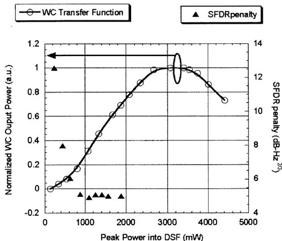
Fig. 5. Calculated SFDR power penalty introduced by the wavelength converter for various points of operation on the transfer function.
