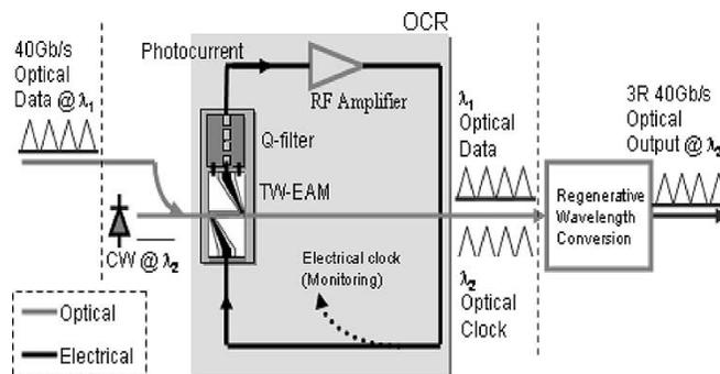
Fig. 1. 3R architecture using the proposed OCR.
