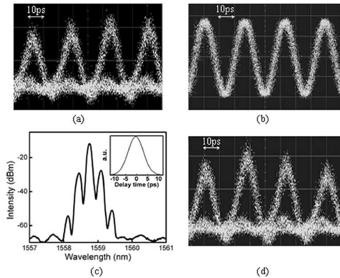
Fig. 4. (a) Eye diagram of  $\sim 40$ -Gb/s input OTDM signal. (b)  $\sim 40$ -GHz generated optical clock and (c) its optical spectrum (resolution bandwidth: 0.1 nm) and autocorrelation curve (inset). (d) Eye diagram of output OTDM signal.
