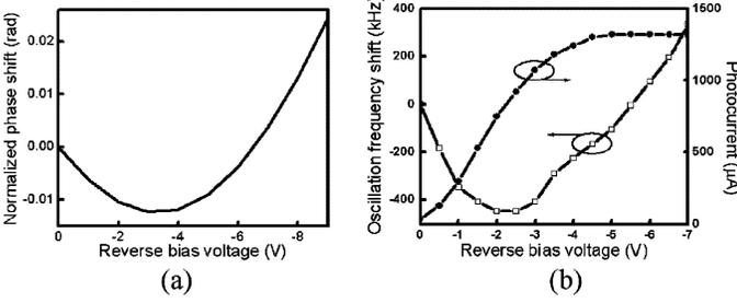
Fig. 2. (a) Simulation result of the relationship between the normalized phase shift and the reverse bias ( $A = -64.11176$ ,  $B_1 = -492.01361$ ,  $B_2 = -42.66419$ ,  $g = 9.9$ ,  $\alpha = 0.1$ ). (b) Measured result of the oscillation frequency shift (square symbol curve) and TW-EAM photocurrent (circle symbol curve).
