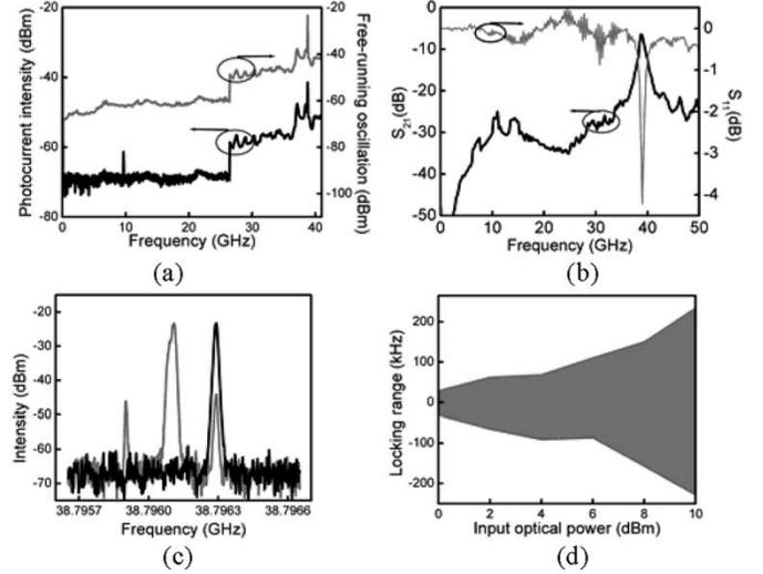
Fig. 3. (a) RF spectra of TW-EAM's photocurrent (lower dark curve) and the OCR free-running oscillation (upper gray curve). (b)  $S$  parameters of 40-GHz  $Q$  filter. (c) RF spectra of noninjection locked (gray line) and injection locked (dark line) optical output. (d) OCR's locking range.
