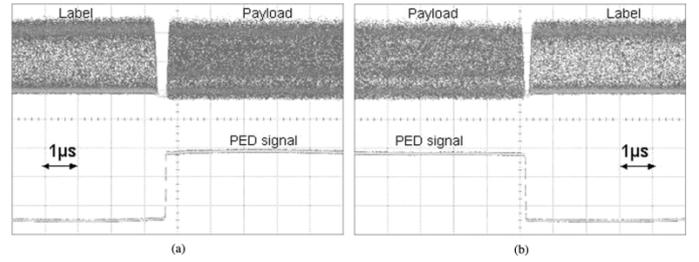
Fig. 3. Zoom in (a) front and (b) rear waveforms of input 40-Gb/s payload and recovered 40-GHz packet clock.
