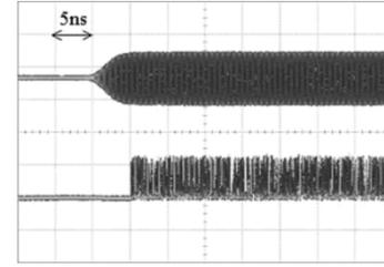
Fig. 4. Oscilloscope traces of the input 40-Gb/s payload (lower) and the recovered 40-GHz packet clock (upper).
