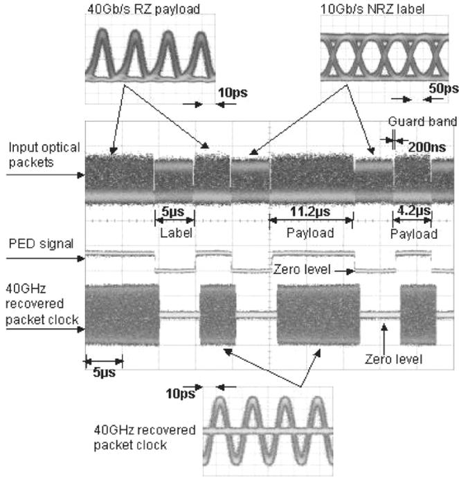
Fig. 2. Oscilloscope traces of the recovered 40-GHz packet clock (lower), the PED signal (middle) detected from the input optical packets (upper). Inset: Corresponding eye diagrams.
