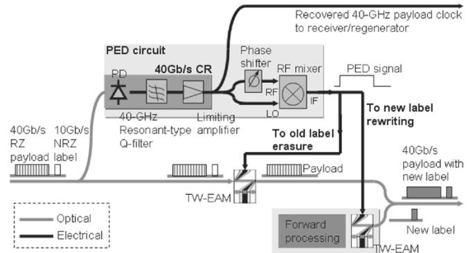
Fig. 1. Scheme of label erasure/rewriting using PED circuits.
