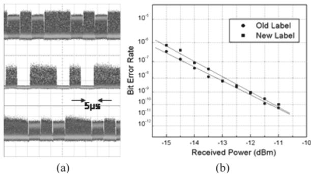
Fig. 6. (a) Demonstration of label swapping: waveforms of old label erasure (middle) and new label rewriting (lower) from the input optical packets (upper). (b) Measured BER results of label erasure and rewriting.
