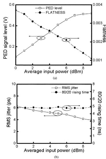
Fig. 5. (a) PED signal level and its flatness and (b) rms jitter and 80/20 rising time of the PED signal against the input average packet power.
