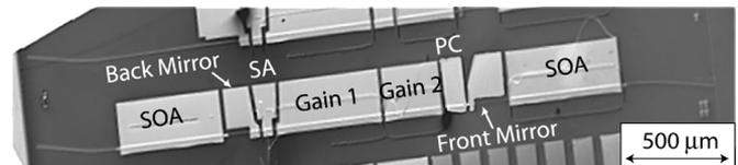
Fig. 1. Scanning electron micrograph of the device.
