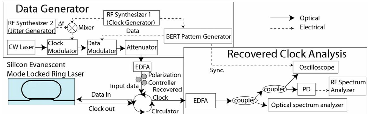
Fig. 2. Experimental setup of the all-optical clock recovery experiments.
