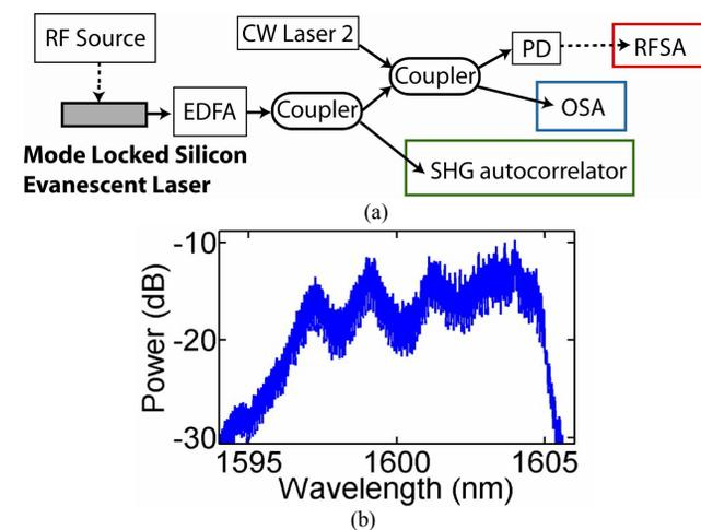
Fig. 1. (a) Experimental setup. (b) Optical spectrum of the 10-GHz ML-SEL with 0.06 nm resolution, which can not resolve the individual modes well.
