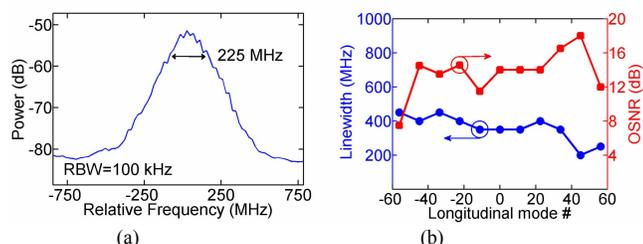
**Fig. 2.** (a) RF spectrum of the CW signal beat together with the ML-SEL output with 100 kHz resolution. (b) OSNR and 3-dB linewidth versus ML-SEL mode number. Mode 0 corresponds to 1600 nm.
