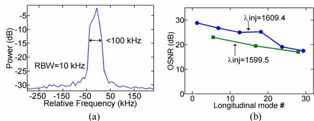
**Fig. 3.** (a) RF spectrum showing the linewidth under CW injection to the ML-SEL at 1609.4 nm, with 100 kHz resolution. (b) OSNR versus mode number for 2 different injected wavelengths. Mode 0 corresponds to the injected CW wavelength.
