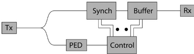
Fig. 4. Experimental setup of synchronously loaded packet buffer.
