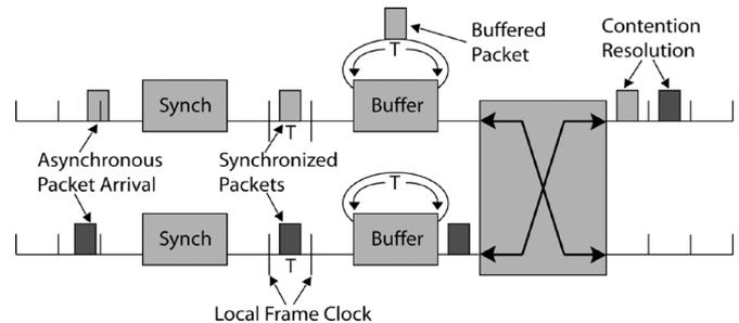
Fig. 1. Packets arrive asynchronously to optical switches. Synchronous buffers align packets to a local frame clock and resolve contention.
