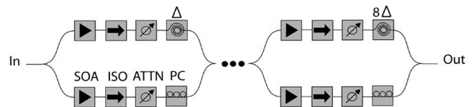
Fig. 2. Fiber-based four-stage synchronizer with SOA gates. (ISO: isolator. ATTN: attenuator. PC: polarization controller.)
