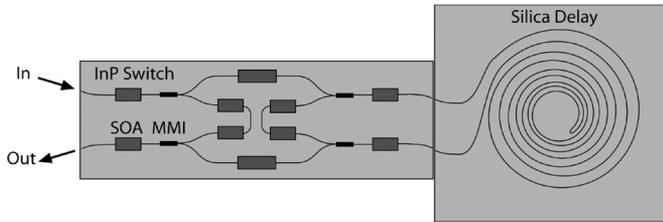
Fig. 3. Integrated buffer with InP switch butt-coupled to 12.8-ns silica-on-silicon delay line. (MMI:  $1 \times 2$  multimode interference splitter.)
