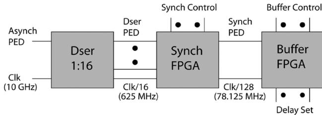
Fig. 5. Electronic control consists of PED, 1:16 Dser, synchronizer FPGA, and buffer FPGA.
