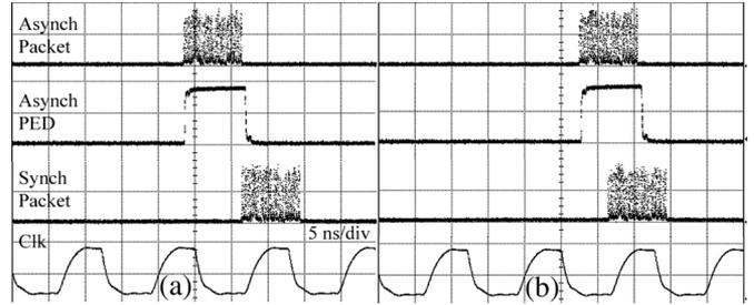
Fig. 6. Screenshots of asynchronous packet arrival, recovered asynchronous PED, synchronized packet, and local clock (a) Synchronizer delay of  $T(10)$ . (b) Synchronizer delay of  $T(5)$ .
