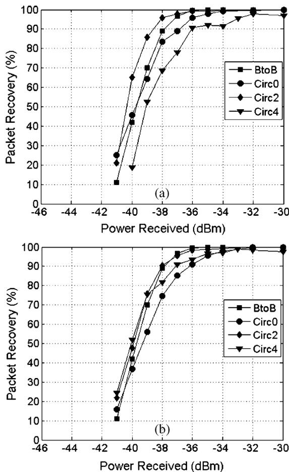
Fig. 8. Packet recovery measurements of synchronous buffer. (a) Synchronizer delay of  $T(10)$ . (b) Synchronizer delay of  $T(5)$ .
