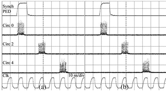
Fig. 7. Screenshots of synchronous PED, buffer circulations of zero, two, and four, and local clock. (a) Synchronizer delay of  $T(10)$ . (b) Synchronizer delay of  $T(5)$ .
